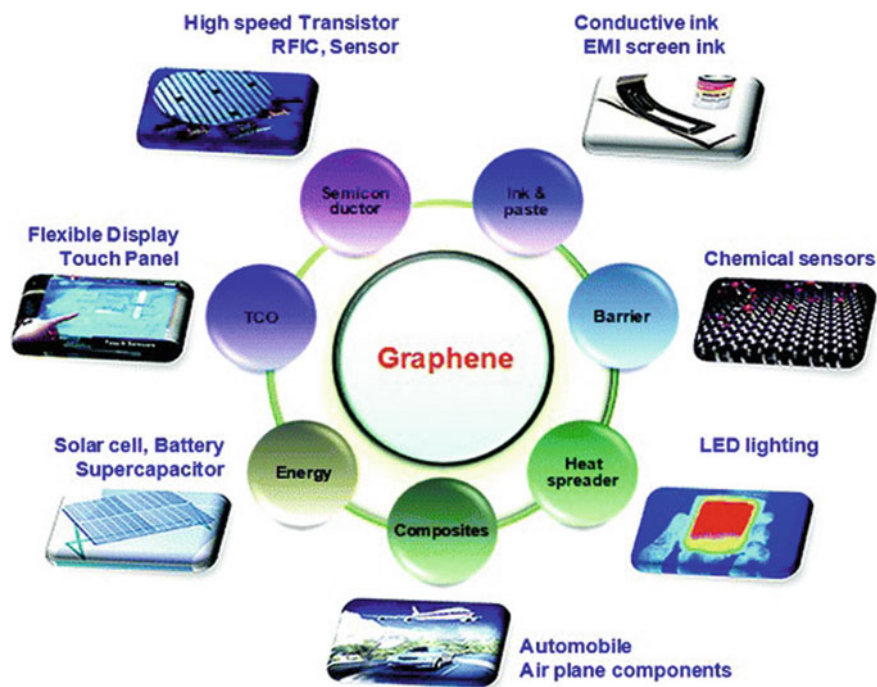
Fig. 3.15 Overview of applications of graphene in different sectors. Adapted with permission from Ref. [92] Copyright (2015) (Royal Society of Chemistry)
