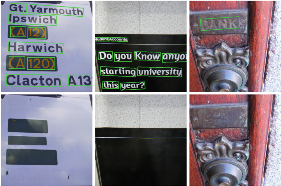
Fig. 1. Examples of scene text removal. Input an image with scene text and text regions, STRDD can remove the text fill with visually plausible content. From left to right, in each example, the top is the input image of IC13 and text regions labeled with polygons in green, while the down is the text-removed images generated by our method
