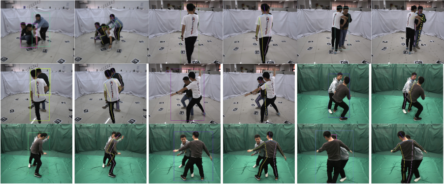
Fig. 3. All images tested are from the Interact-Pose dataset. (a), (c), (e) are the bounding-box of the human body detected in the DCPose algorithm; (b), (d), (f) are the results of the pose estimation; if there is a missing bounding-box detection, or the detection result of the bounding-box is not accurate enough, which will have a great impact on the subsequent human pose estimation results.
