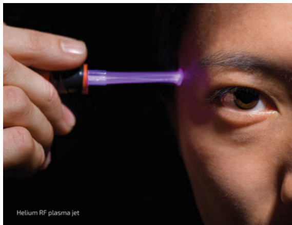
Fig. 1.2 DBD-based atmospheric pressure plasma jet interacting with skin
