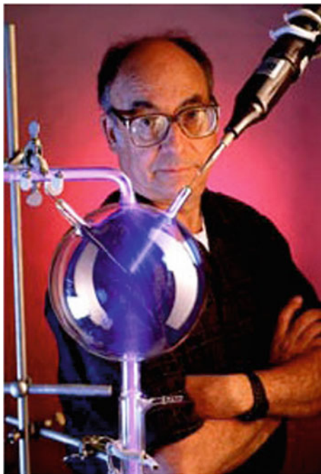
Fig. 1.3 Stanley Miller from University of Chicago in 1950s produced amino acids using inorganic compounds and methane with plasma
