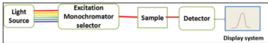
Fig. 15.19 Schematic diagram of key components in a UV-vis spectrometer
