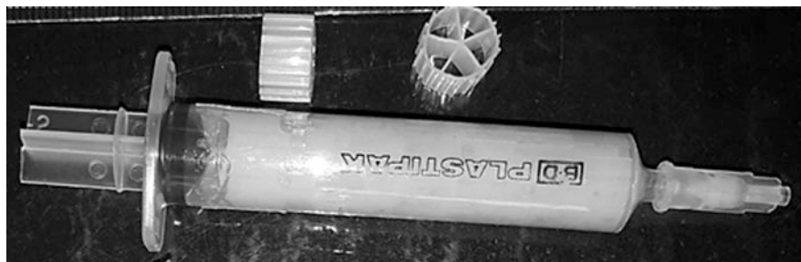
Fig. 1.9 Kaldnes carriers (at the top) and cryogels with immobilized bacteria prepared in Kaldnes carriers in the syringe (at the bottom)
