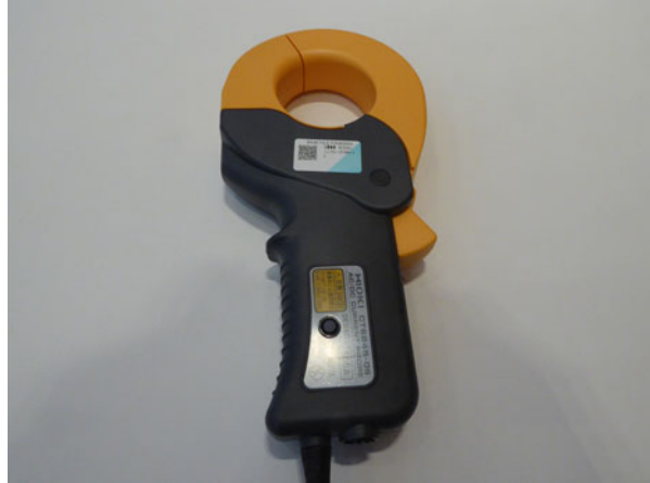
Fig. 6.12 Example of a clamp-type current probe used for GIC observations
