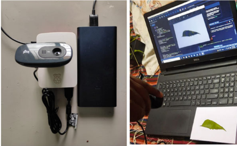
Fig. 10 Hardware Implementation and capturing image using webcam
