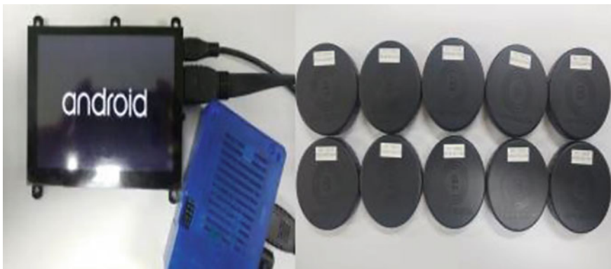
Fig. 2 Odroid-C2 (L) and Onyx Beacon One (R) used for app. function test
