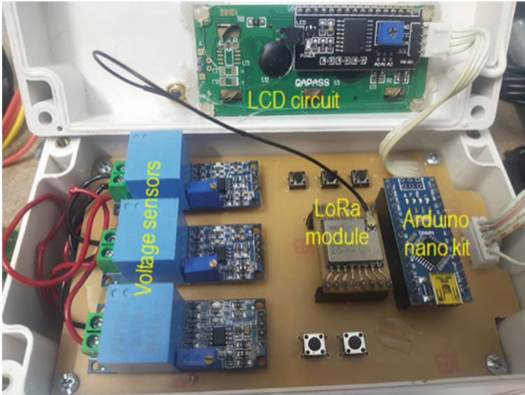
Fig. 7 Electronic circuits of the sensor nodes
