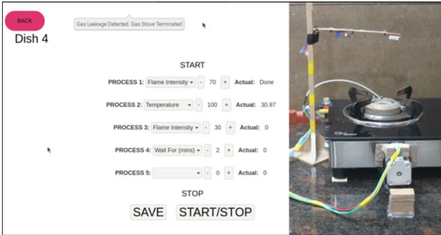
Fig. 9 Experimental setup of gas automation module to test for gas leakage
