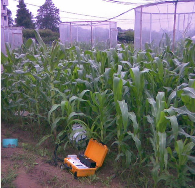
Fig. 7 LI-8100 system along with short-term survey chamber to obtain soil CO 2 flux (Source: Daripa, 2009)
