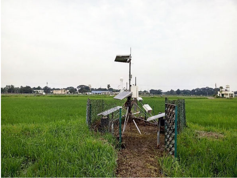
Fig. 6 Eddy covariance system installed at a lowland paddy field of ICAR-NRRI, Cuttack, with CO 2 /H 2 O analyzer (open-path infrared gas analyzer), covering a fetch area of 2.25 hectares, attached with sonic anemometer, temperature-humidity sensor, radiation sensor, and soil temperature probe, connected to a built-in data-logging facility. (Source: Authors' personal collection)
