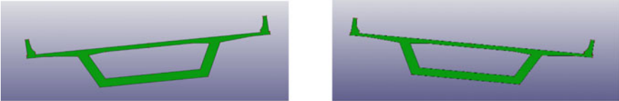
Fig. 4 Bridge deck with no modification subjected to wind attacking angle at 7^\circ
