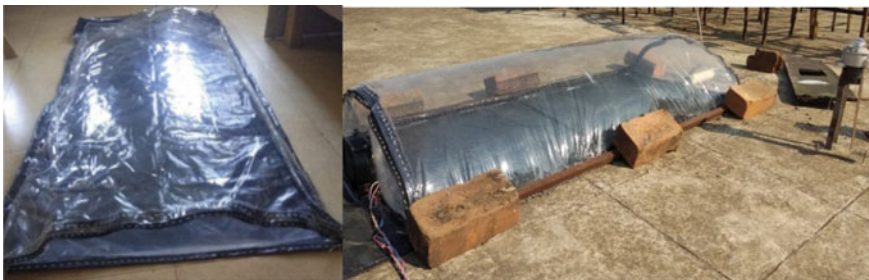
Fig. 1 Developed model of solar bubble dryer (SBD) without inflation and with inflated state
