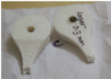
Fig. 4 Pattern of breaking during the load determination for specimen A (a), specimen B (b) and specimen C (c)
