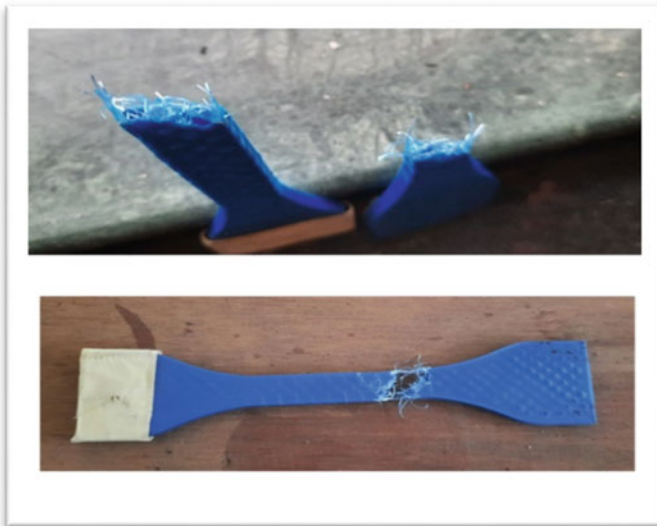
Fig. 4 Failure of specimen from recycled filament
