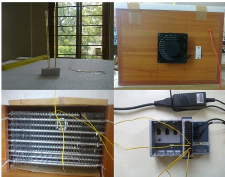
Fig. 3 Different components of experimental test rig (ordered from top left corner in clockwise direction, a dry and wet bulb thermometers, b fan with regulator, c data acquisition system and d front view of evaporator coil)
