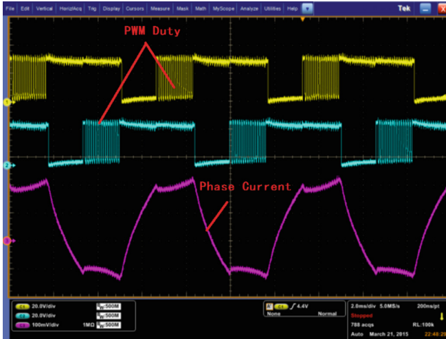
Fig. 10. 50% fixed duty cycle phase current waveform.
