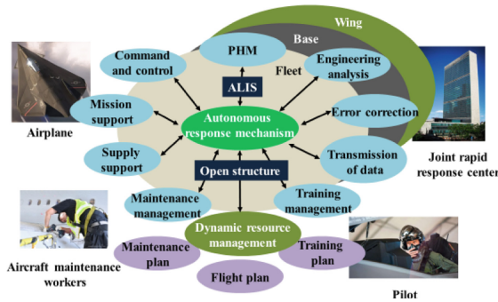
Fig. 2. The F-35 concept map of autonomic support [16]
