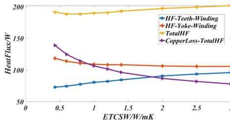
Fig. 5. Heat flux variation with ETCSW
