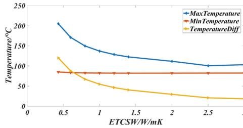
Fig. 6. Winding temperature variation with ETCSW
