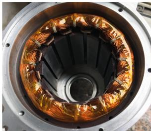
**Fig. 1.** Slot winding of an electrical aviation machine
