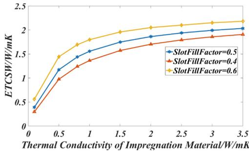
**Fig. 2.** Equivalent thermal conductivity of the slot winding
