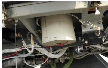
Fig. 13. Actuator in a light helicopter [21].
