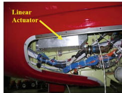
Fig. 12. Linear actuator on Bell 429 [5].
