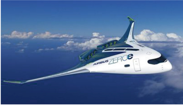
Fig. 12. The blended wing body passenger aircraft concept scheme of ZEROe
