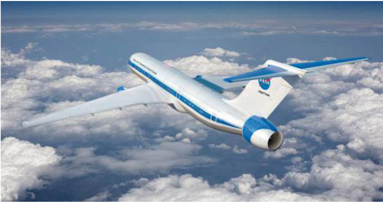
Fig. 1. The single-aisle turboelectric aircraft with aft boundary layer of NASA
