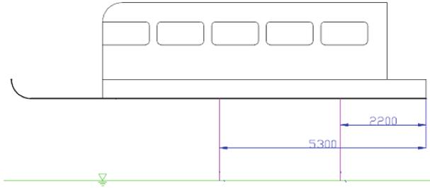
**Fig. 2.** Longitudinal position schematic diagram of air flow field measurement point
