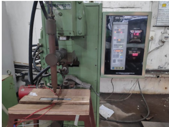
Fig. 1 Spot welding machine (KEJE make) used for experimentation
