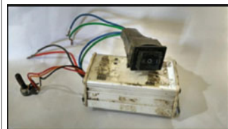
Fig. 2 a First prototype of clay 3D pen and b clay 3D pen with changes in the prototype
