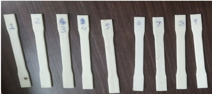
Fig. 1 Specimen as per ASTM standard D 638 Type IV
