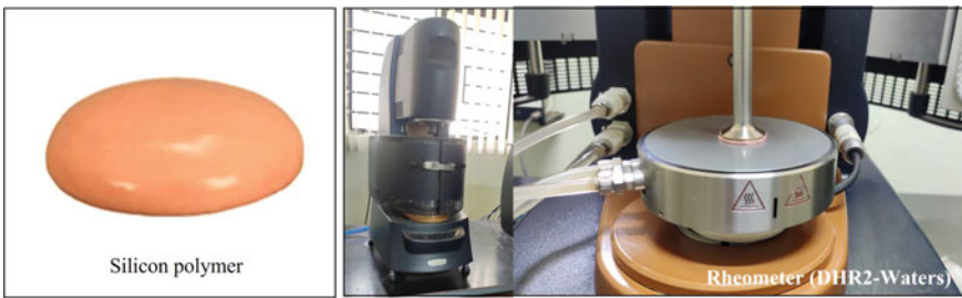
Fig. 1 Viscoelastic polymer media analysis through rheometer (DHR2-waters)
