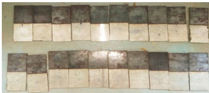
Fig. 2 Samples of joints produced by CO 2 LBW experiments
