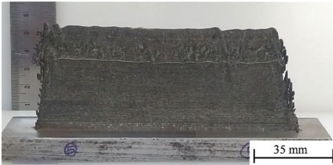
Fig. 9 Wall with mitigated waviness (212 layers)
