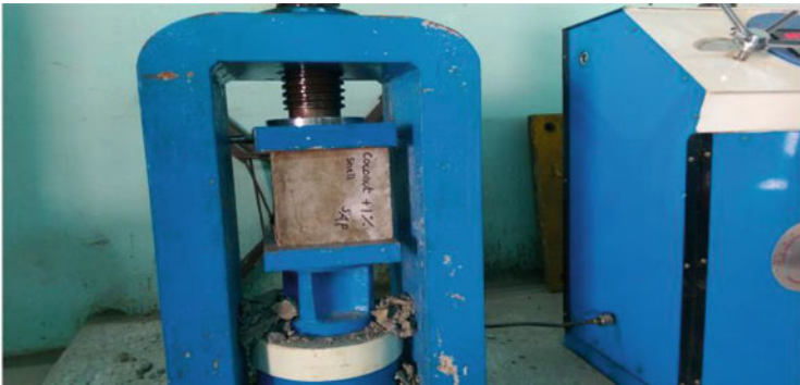
TEST SET UP – COMPRESSIVE STRENGTH
