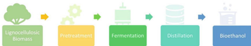
Fig. 11.1 Bioethanol production process flow
