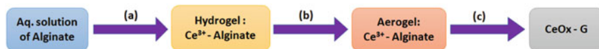
Fig. 7.2 Process for the preparation of \text{CeO}_x/\text{G} nanocomposite: (a) precipitation of the alginate hydrogel containing \text{Ce}^{3+} with (\text{NH}_4)_2\text{Ce}(\text{NO}_3)_6 ; (b) drying by \text{H}_2\text{O} to EtOH exchange followed by supercritical \text{CO}_2 drying; and (c) pyrolysis under argon flow
