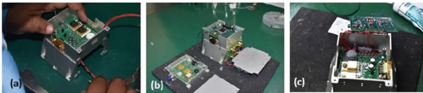
Fig. 5 Photographs of RFMEMS-TD1 at various stages of assembly a power module integration b RF module assembly c FPGA card assembly into the housing
