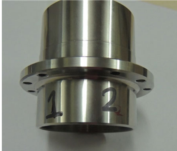
Fig. 5 Bearing unit housing used for test
