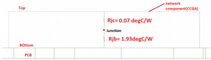
Fig. 1 Network block defines CCGA (thermal resistance from junction to top is less hence heat flow to the top)
