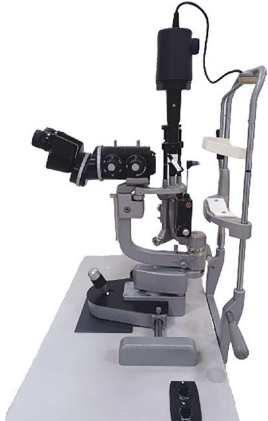
Fig. 4.5 Slit lamp-mounted Goldmann applanation tonometer (Haag Streit, USA)
