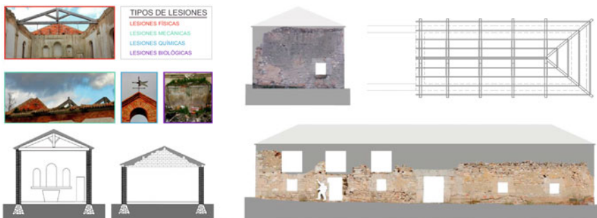
Fig. 7.5 Students' works: constructive pathology and preliminary project planimetry
