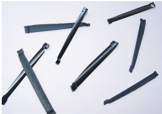
Fig. 1. The geometry of mill cut steel fibers
