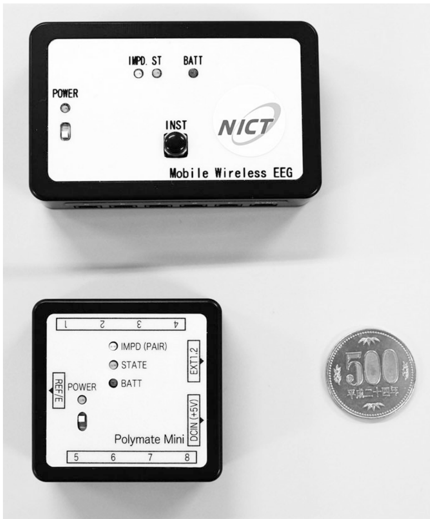
Fig. 12.3 Upper: prototype of the electroencephalography (EEG) device. Lower: commercialized EEG device manufactured by MIYUKI GIKEN
