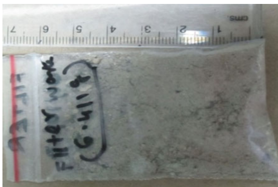
Fig. 8 Morphology of filter residue after air plasma treatment
