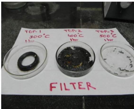
Fig. 5 Morphology of residue after treatment with resistance heating
