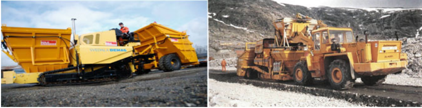
Fig. 29.4 Asphalt core placing machine (paver) [4]
