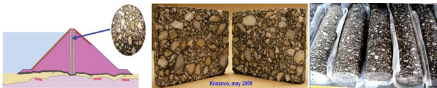
Fig. 29.7 Typical image of asphaltic core concrete [8]
