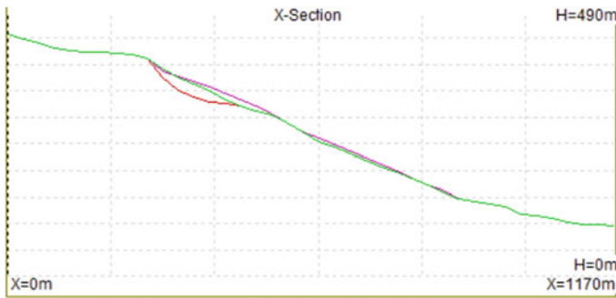
Fig. 23.3 Sliding surface in longitudinal section of soil slope situated at Kakkattuppara region subjected rainfall intensity with PPR of 0.7
