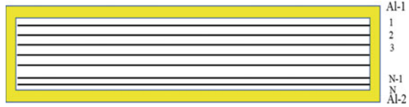
Fig. 3 PCM layers encapsulated aluminium base
