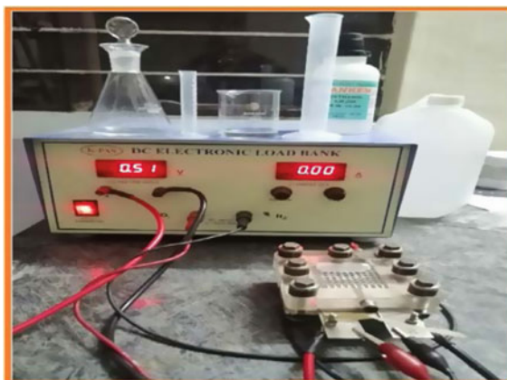
Fig. 3 Experimental set-up of passive DMFC
