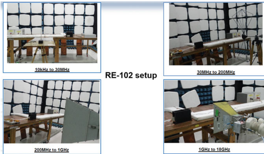
Fig. 6 RE102 test setup
