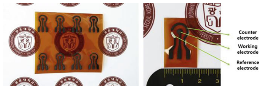
Fig. 3 LIG electrode on PI film (125 \mu\text{m} in thickness). Reprinted with permission from reference Park et al. [25]. Copyright 2020 Elsevier
