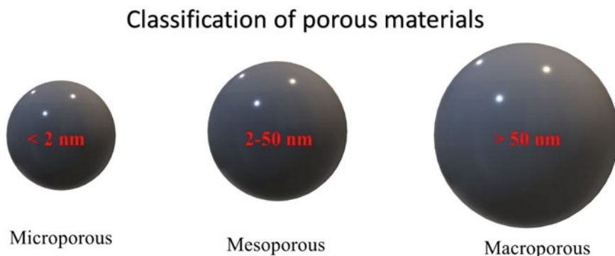
Fig. 2 Classification of porous materials based on pore diameter
