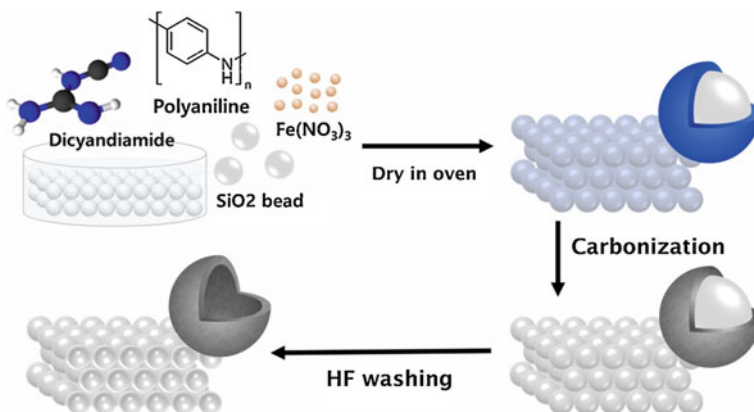
Fig. 4 Schematic illustration of the procedure of the synthesis of porous doped carbon nanostructures. Reprinted with permission from Kwon et al. [62]. Copyright 2019 The Korean Society of Industrial and Engineering Chemistry. Published by Elsevier B.V
