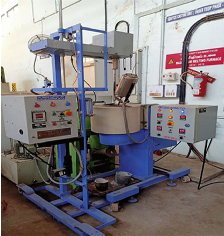
Fig. 1 Stir casting setup
