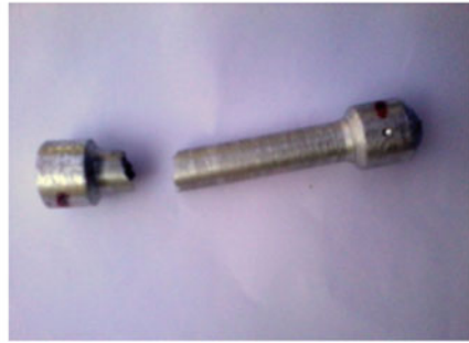
(c) Specimens after tensile test
