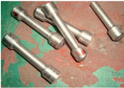
(b) Specimens before tensile test
