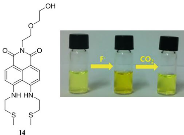
Fig. 12 Structure of Naphthalimide derivative (Left) and colour change displayed by sensor 14 by interacting with F^- and CO_2 (Right) (adapted from references [18])
