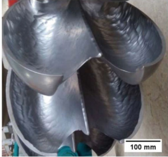
Fig. 2.8 Eroded Pelton Bucket of Toss H.P.P. (Rai et al. 2017)
