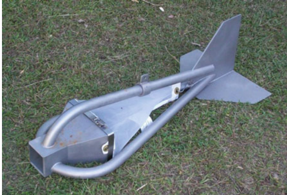
Fig. 2.16 Pressure difference type bed load sampler (Erskine et al. 2011)
