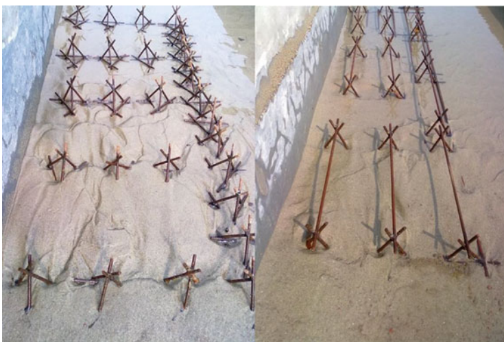
Fig. 17.3 Experimental flume with triangular and prismatic porcupine fields
