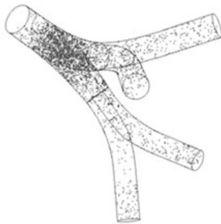
Figure 5. Locations of particles in airway with 2\mu\text{m} diameter for the case U_1 .
