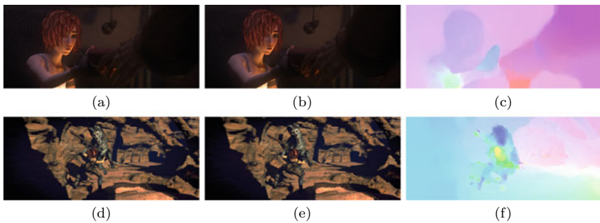
Fig. 3.7 Examples of flow estimation in MPI-Sintel test set. a frame_0024 and b frame_0025 of sequence PERTURBED_shaman_1. c estimated optical flow for sequence PERTURBED_shaman_1. d image frame_0041 of sequence tiger1. e image frame_0042 of sequence tiger1. f estimated optical flow for sequence tiger_1
