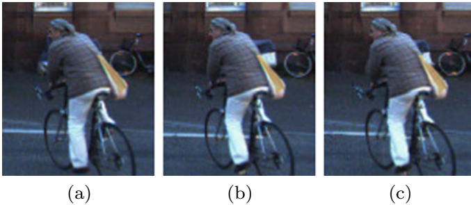
Fig. 3.2 Creation of an image in between. a Current image. b Next image. c Image in between created based on optical estimation
