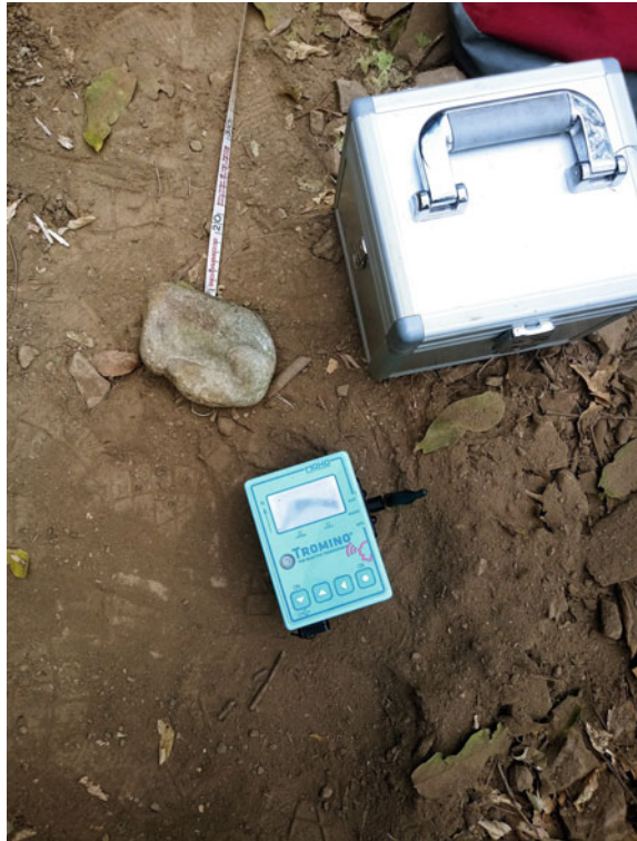
Fig. 34.2 Microtremor testing equipment (TROMINO®) setup in the field
