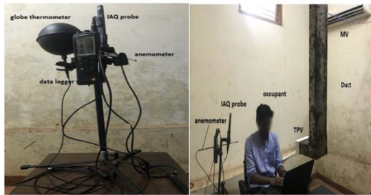
Figure 4: Instrument details and measurement methods
