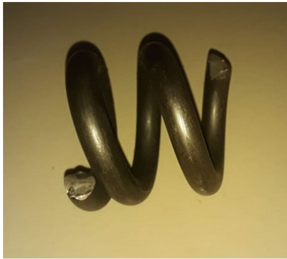
Fig. 10 Failed helical suspension spring
