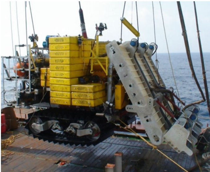
Fig. 4 Polymetallic module mining under qualification (Vedachalam et al. 2018)
