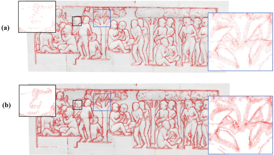
Fig. 5. Edge-highlighting visualization of the relief panel of Fig. 4. (a) shows the edge-highlighting visualization based on the original opacity-based edge highlighting [1]; (b) shows the edge-highlighting visualization based on our method.
