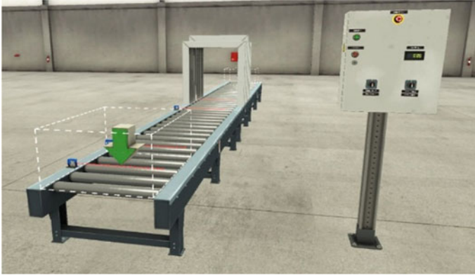
Fig. 10 Automated disinfection in factory IO of polyethylene terephthalate bottles for bacteria, fungi, and viruses; by UVC LED camera
