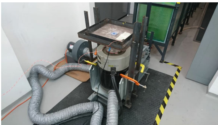
Fig. 3 Impact vibrator with the test panel placed on the top
