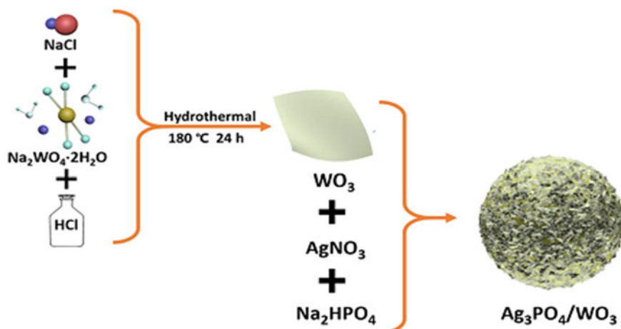
Fig. 22 Synthesis route of \text{Ag}_3\text{PO}_4/\text{WO}_3 heterojunction (Copyright Elsevier License Number 5319270917223)
