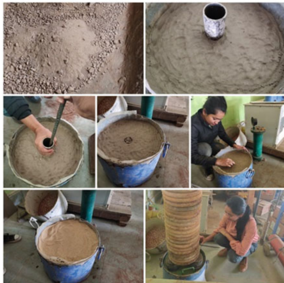
Fig. 12.2 Preparation of soil bed and stone column
