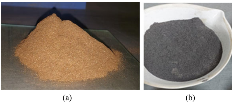
Fig. 34.1 Materials used in the study a sawdust b sawdust ash
