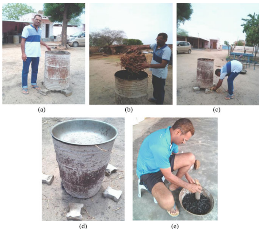
Fig. 24.1 a Cylindrical drum used for making biochar; b filled with crop residues; c set to fire at the bottom; d The supporting bricks removed from the bottom and top is covered with a lid; biomass is allowed to heat inside for 10–15 min; and e raw biochar is crushed into pieces
