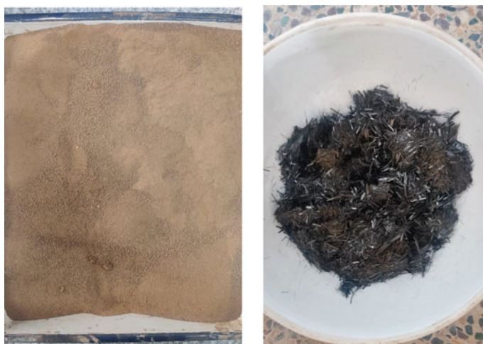
Fig. 28.1 Soil and the carbon fibers used in the present study
