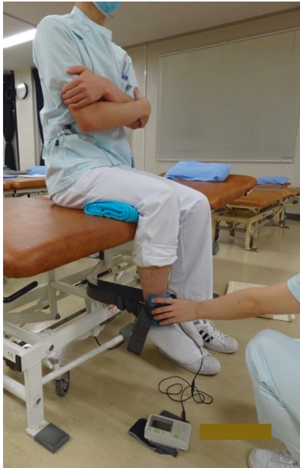
Fig. 4.2 Hand-held dynamometers (HHDs) are used to measure knee extensor muscle strength as an index of lower-limb muscle strength
