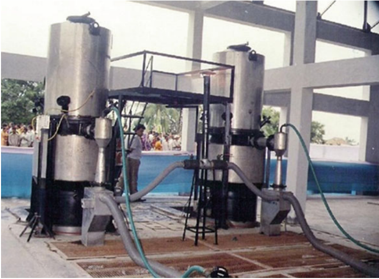
Fig. 8 500 KWp Chhoto Mollakhali biomass gasifier power plant [19]
