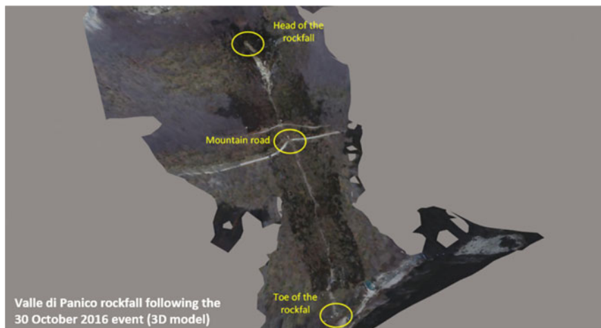
Fig. 16 sUAS-based 3D model of the Valle di Panico rockfall (modified from GEER 2017)
