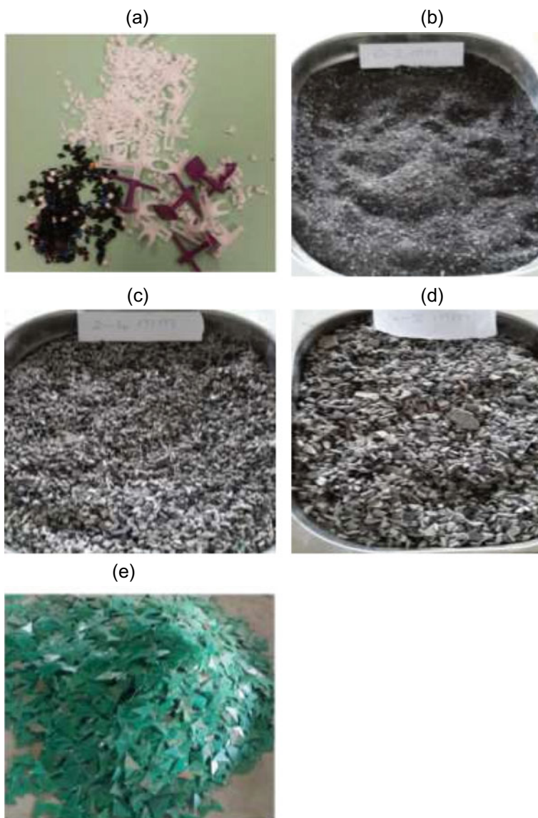
Fig. 1 Varying particle sizes of e-plastic waste aggregates; a chopped/grounded/shredded e-plastic aggregate (Mills and Tatar 2016); b E-plastic of size 0–2 mm (Bulut and Şahin 2017); c E-plastic of size of 2–4 mm (Bulut and Şahin 2017); d E-plastic of size 4–8 mm (Bulut and Şahin 2017); and e E-plastic of size 20 mm (Shinu and Needhidasan 2020)
