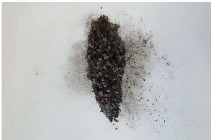
Fig. 1 Electroactive components isolated after elimination of the non-aqueous solvent and manual scraping
