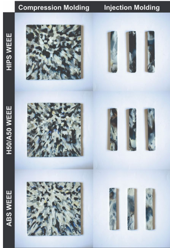
Fig. 6 Samples of HIPS WEEE, H50/A50 WEEE, and ABS WEEE obtained by compression
