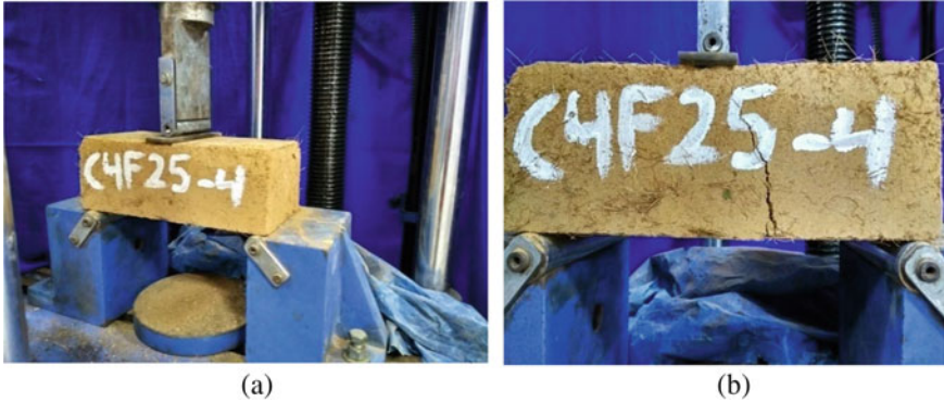
Fig. 1.3 Blocks under flexure loading: a before test and b after test
