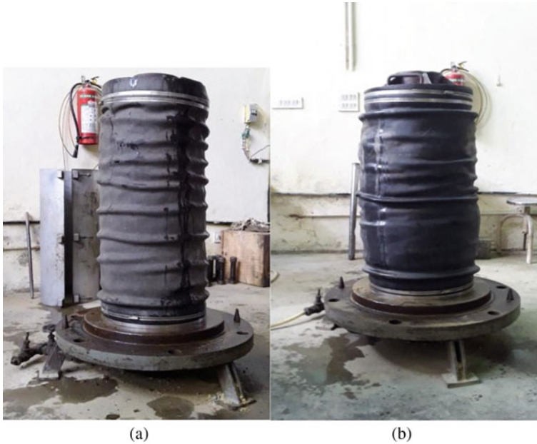
Fig. 8.1 After the test, observation the pattern of failed specimen. a 25 mm particle under 0.6 MPa confining pressure. b 80 mm particle under 1.8 MPa confining pressure
