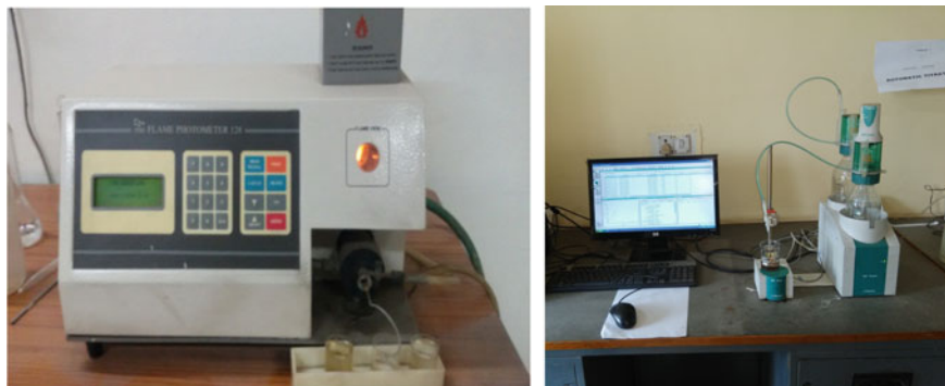
Fig. 3.2 Determination of sodium and potassium in pore water extract with flame photometer and determination of chloride with automatic titrater
