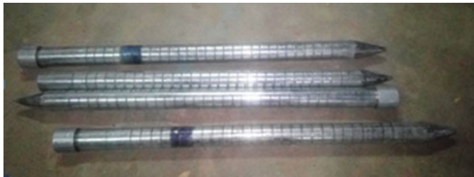
Fig. 19.6 Typical photograph showing laterals with collars and sharp driving edge
