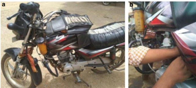
Fig. 3 a and b Mileage testing bottle is being attached on two-wheeler
