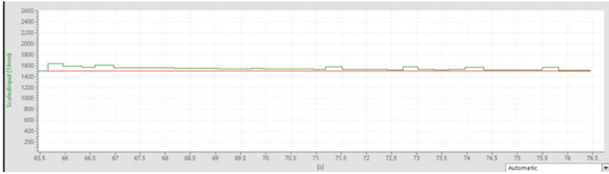
Fig. 12 Generator 1: decrease from full load by no load
