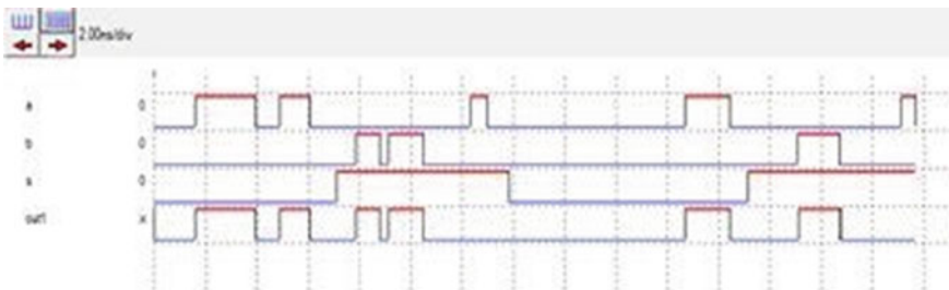
Fig. 8 Simulated waveform of 2:1 MUX using ECRL
