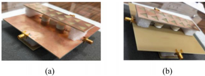
Fig. 8 Fabricated antenna structure; a top view; b bottom view
