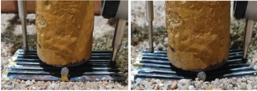
Fig. 18.3 Deformation of footing during application of load
