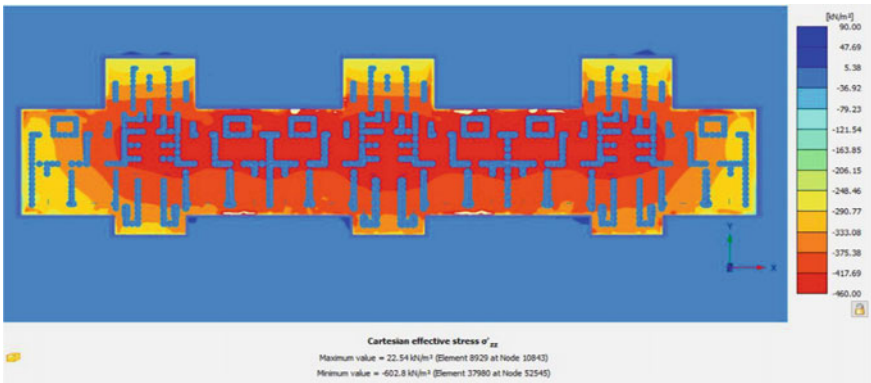
Fig. 9.11 Pressure contours at soil–raft interface
